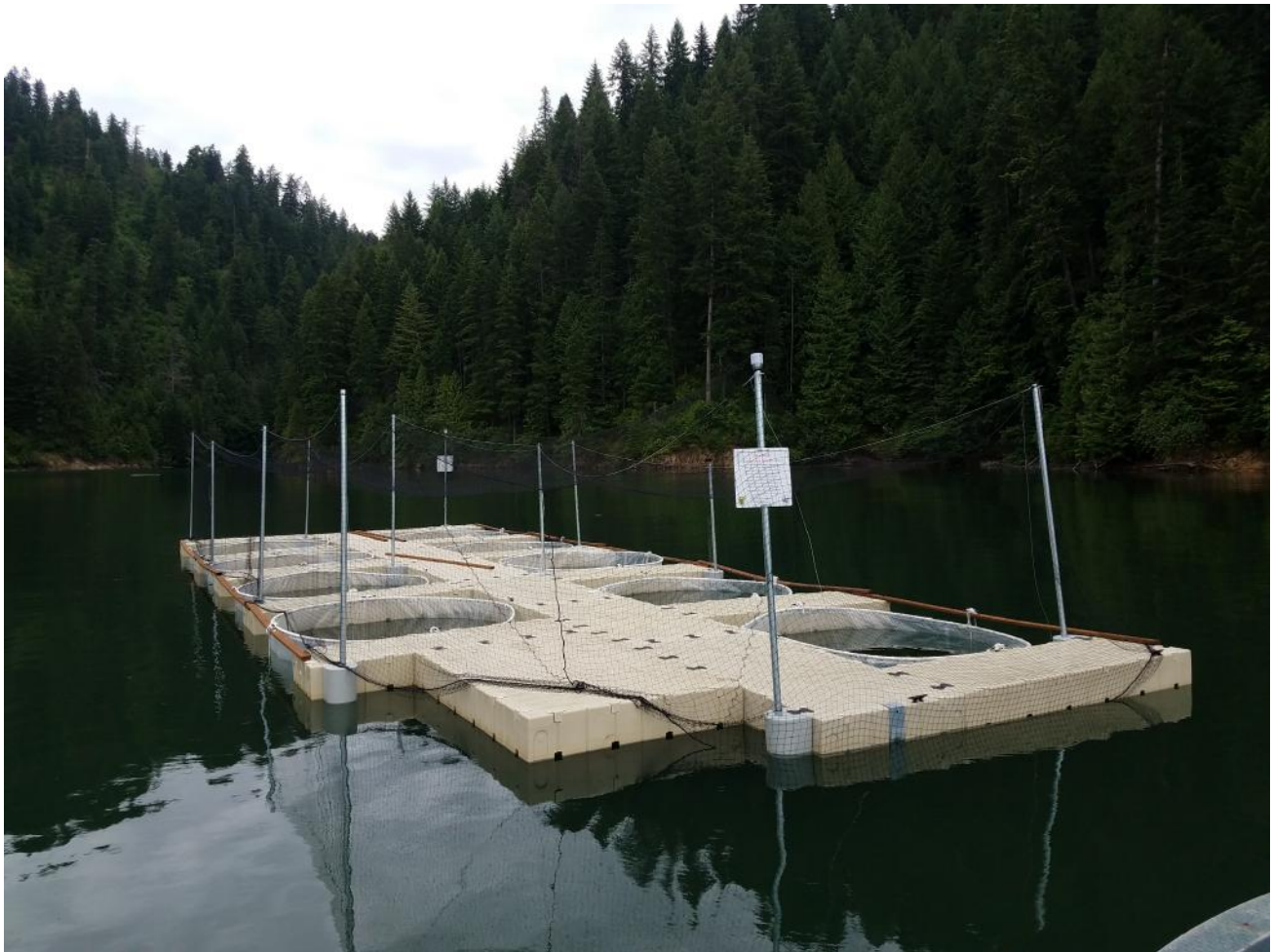
The docks and experimental enclosures near the mouth of Hodson Creek used to study nitrogen addition. Reservoir users are asked not to use the dock or disturb the enclosures.
