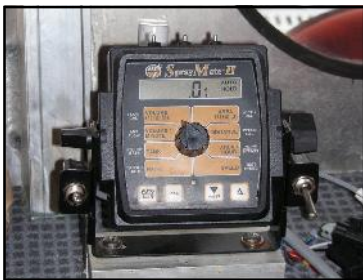
GPS linked application controller
