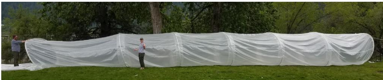
A 65 foot long plastic enclosure stretched out horizontally on the ground prior to deployment in the reservoir. Enclosures were suspended vertically into the water to enclose a portion of the water column to test the effects of nitrogen addition.
